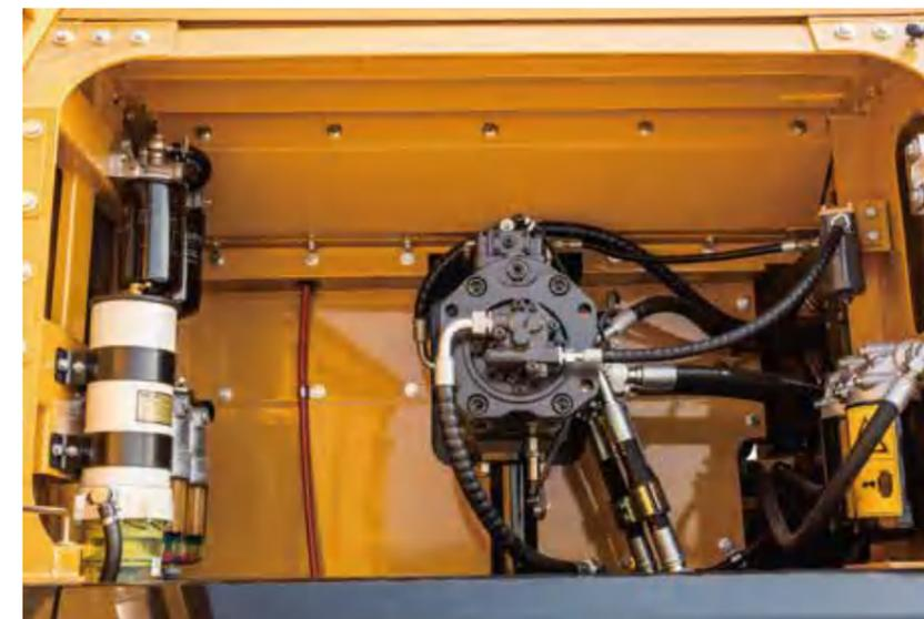
High-capacity multi-stage filter system
