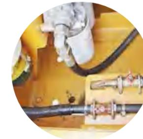
Water drain valve of fuel tank
