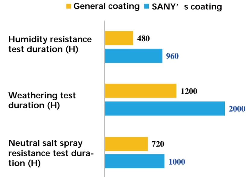
Coating distribution of SANY' s high corrosion-resistant paint
