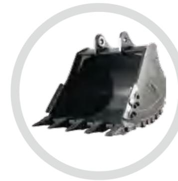
Motion trail of bucket bottom is optimized, excavation resistance is reduced, excavating speed is increased, working efficiency is improved by 10%. High-strength wear-resisting steel plate is used and bucket wear-resisting performance is improved by 2 times. With professional bucket design for stonework, it is more suitable for heavy-duty operation like quarry etc.
