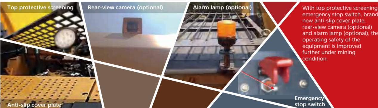
With top protective screening, emergency stop switch, brand new anti-slip cover plate, rear-view camera (optional) and alarm lamp (optional), the operating safety of the equipment is improved further under mining condition.
