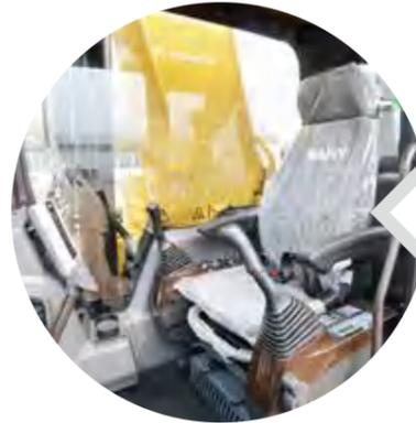
The FOPS/ROPS cab is adopted, and through finite element modal analysis, the steel structure and sealing property of cab are optimized, so that its strength is 5 times that of ordinary cab and the safety is improved; the high-power air conditioning system is provided, so that the refrigerating and heating effect can be achieved quickly and the driving/riding will be more comfortable.
