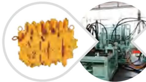
With pump-valve endurance test bed, the service life of main pump and main valve are tested and analyzed. In combination with research achievements of long-life parts of the customer, the service life of the pumps and the valves is improved by 1 time.
