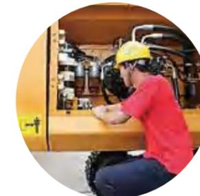
Replace diesel oil filter element
